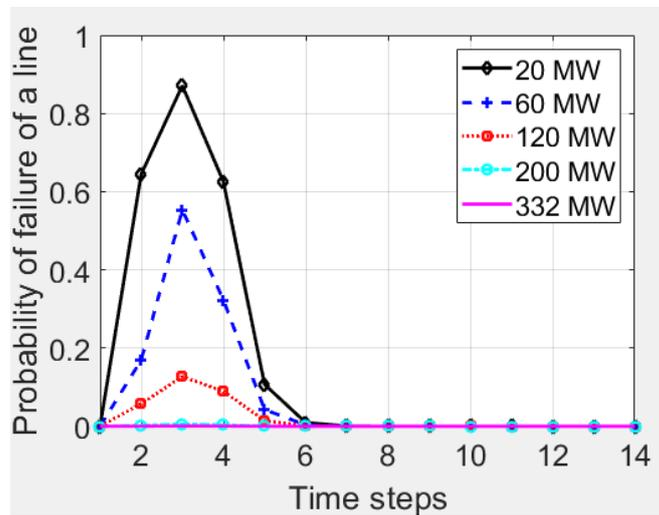
Figure-7: Probability of failure of a line with time step
