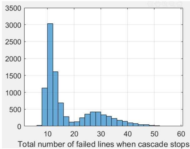
Figure-3: Number of failed lines
