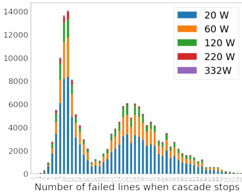
Figure-5: Number of failed lines in each category at steady state
