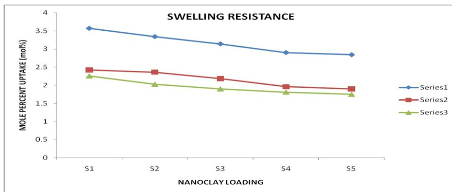
Figure 8.6 Swelling resistance (in terms of mole percent uptake) of the EPDM/NBR composites: Series 1 (Toluene solvent), Series 2 (pentane solvent) and Series 3 (carbon tetrachloride)
