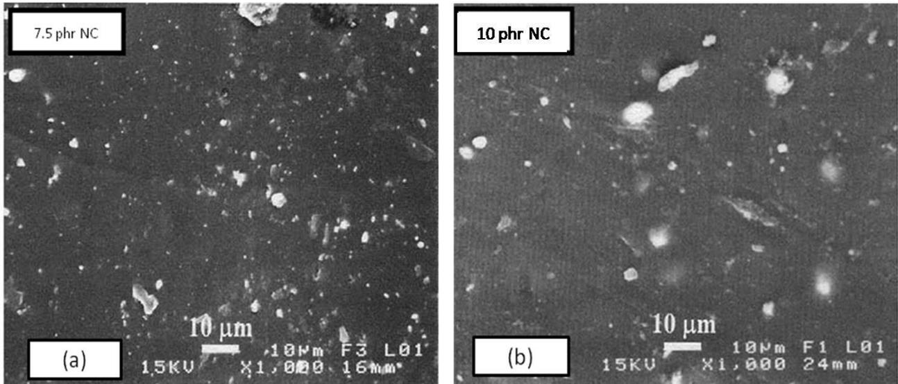
Figure 8.7 SEM micrographs of EPDM/NBR composites
