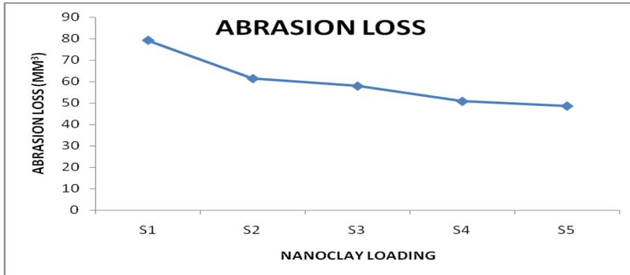
Figure 8.5 Abrasion loss of the EPDM/NBR composites
