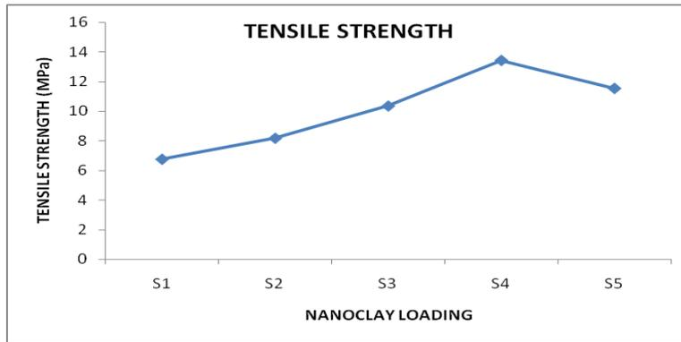
Figure 8.1 Tensile strength of the EPDM/NBR composites
