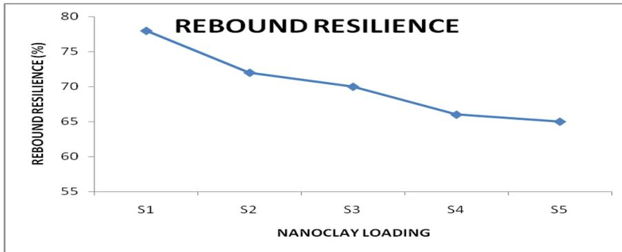
Figure 8.4 Rebound resilience of the EPDM/NBR composites
