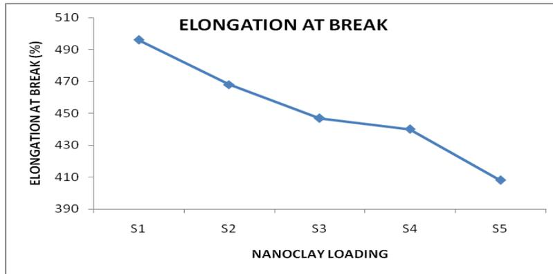
Figure 8.2 Elongation at break of the EPDM/NBR composites
