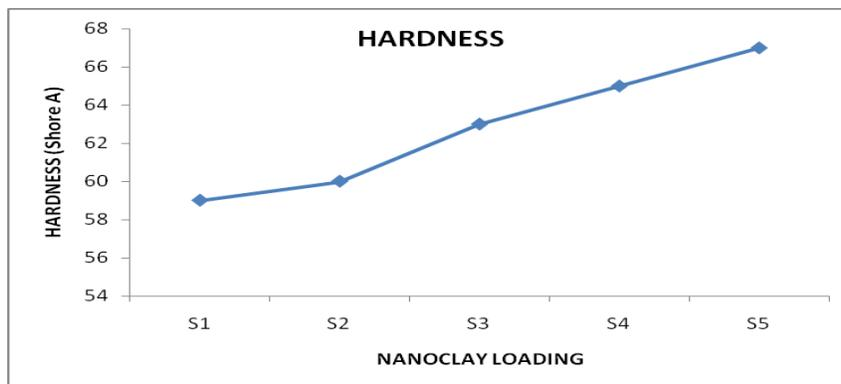
Figure 8.3 Hardness of the EPDM/NBR composites
